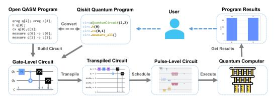
**Figure 4:** Example of process for running quantum circuits on superconducting quantum computers in Qiskit.
