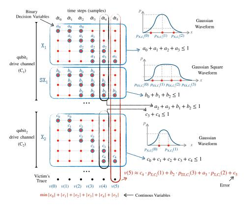
Figure 10: MILP encoding method over an pulse information.
