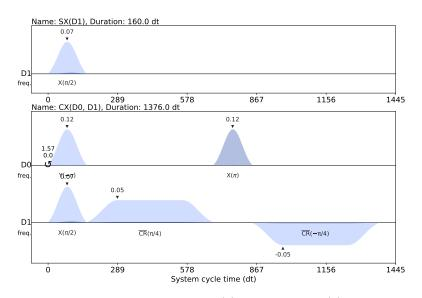
**Figure 9:** Example pulse schedules of SX:  $d_1$  ( $\star$ ) and CX:  $d_0$ - $d_1$  ( $\circ$ ), whose durations are 160dt and 1376dt respectively. As seen from the figure, the first waveform on the drive channel  $d_1$  of CX is exactly the same pulse as in SX.
