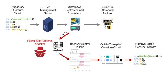
**Figure 1:** Typical operation of a cloud-based quantum computer. Red arrows highlight potential power trace threats.
